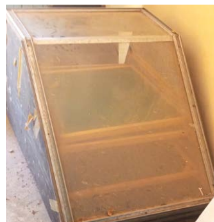
FIGURE 12C: A FOOD SOLAR DRYER
