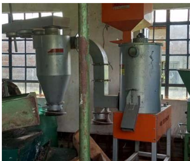
FIGURE 8A AGRO PROCESSING MACHINES INCLUDING DESTONER FOR REMOVING ALL STONE AND METALLIC PARTICLES AND A GRADER FOR GRADING FOOD PRODUCTS SUCH AS COW PEAS, MILLET, GREEN GRAMS AND SORGHUM CEREAL
